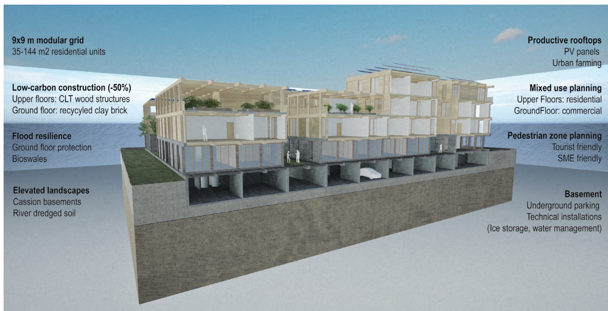
Figure 7. Perspective view of the Lingnan-inspired cluster typology, showing the vertical stratification of flood-resilient base structures (recycled clay brick), cross-laminated timber residential floors, and productive rooftop landscapes Abbreviations: PV: Photovoltaic; SME: Small- and medium-sized enterprise. Source: Diagram by the authors
