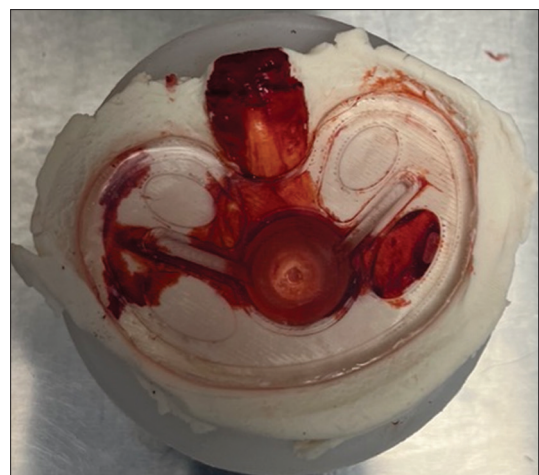
Figure 7. A baseplate trial demonstrating the filling of a cementation pocket with fluid
