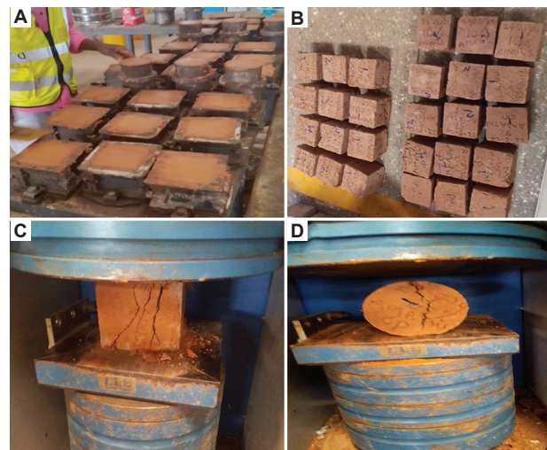
Figure 2. Preparation and testing of specimens: (A) molding of specimens, (B) cube specimens, (C) compressive strength test setup, and (D) tensile strength test setup
