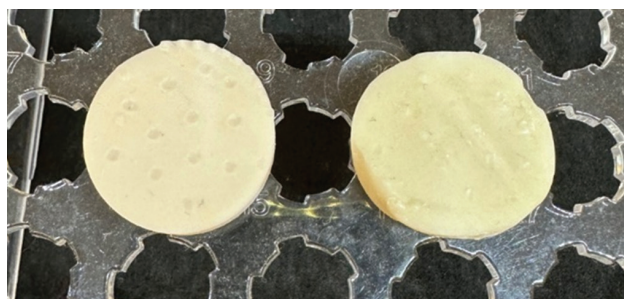
Figure 6. Resin with diacrylate diluent printed coral plug (on the left) and resin without diacrylate diluent printed (on the right).
