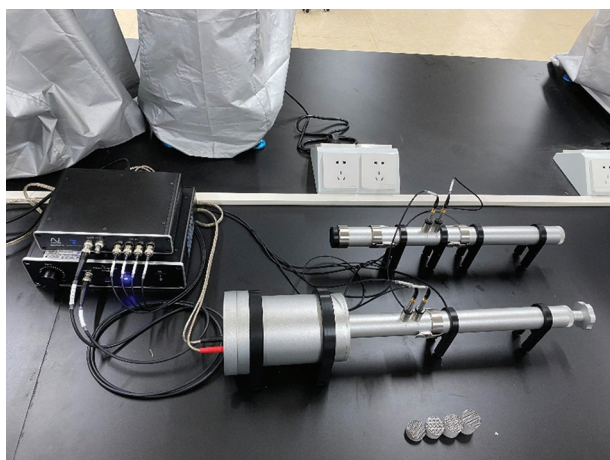
Figure 6. A two-microphone impedance tube
