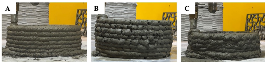
Figure 5. Number of buildable layers before failure for different printable concrete mixes. (A) Control mix for 7 layers; (B) BC5 mix for 9 layers; and (C) BC10 mix for 6 layers.
