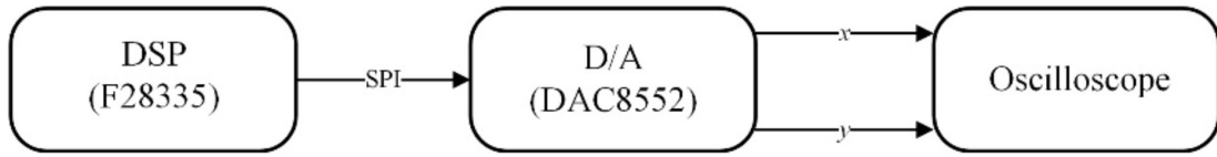
Figure 14. DSP steps and connection diagram Abbreviations: D/A: Digital-to-analog converter; DSP: Demand-side platform; SPI: Serial peripheral interface.
